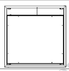
Press and release at the given position from both sides at the same time to unlock the push latches as shown in the figure.
