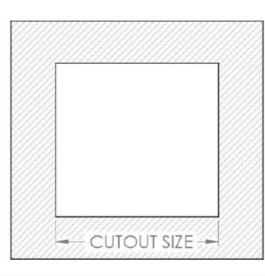
Measure the cutout lengths from the outer frame or by the below mentioned formula and the generate the slot in the exising ceiling accordingly.
