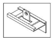
Place the outer frame in the cutout and check for any misalingnment.
